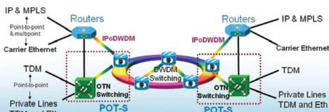
Figure 1: Next Generation Transport Architecture As IP becomes the predominant traffic type, integrated optics on routers (IPoDWDM: IPIMPLS/EthernetDWDM) is the most efficient way to interface with DWDM or a POT-S platform (which supports DWDM, OTN, Ethernet). POT-S can also support private line point-to-point services.
