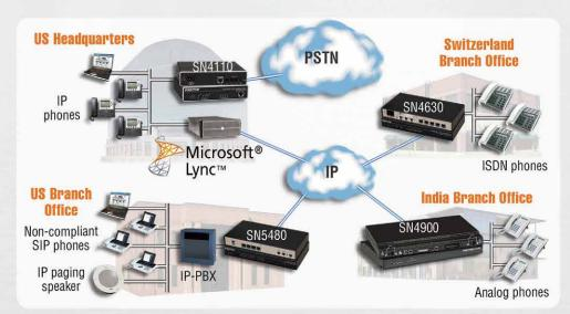
ow any enterprise can reap the benefits of unified communications (UC) with Microsoft Lync. Certified by the Microsoft UC Open Interop Program for Lync server, Patton's SmartNode<sup>™</sup> products provide the "gateway to Lync" for your office communications equipment and software—certified or not.
